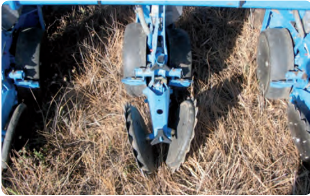
Fig. 3.21. Detail of row closure using double disc.
