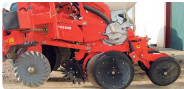
Fig. 3.19. Sowing train in a single grain planting machine.
