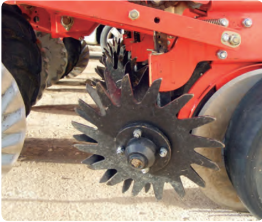
Fig. 3.16. Stubble sweeper mounted on the sowing train.
