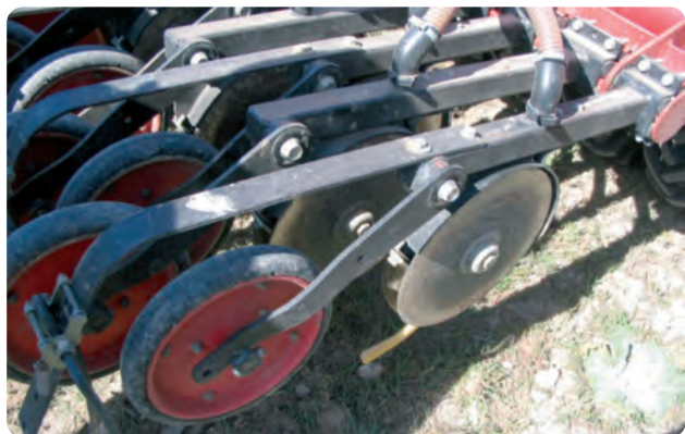
Fig. 3.18. Seed drill equipped with double disc opener.
