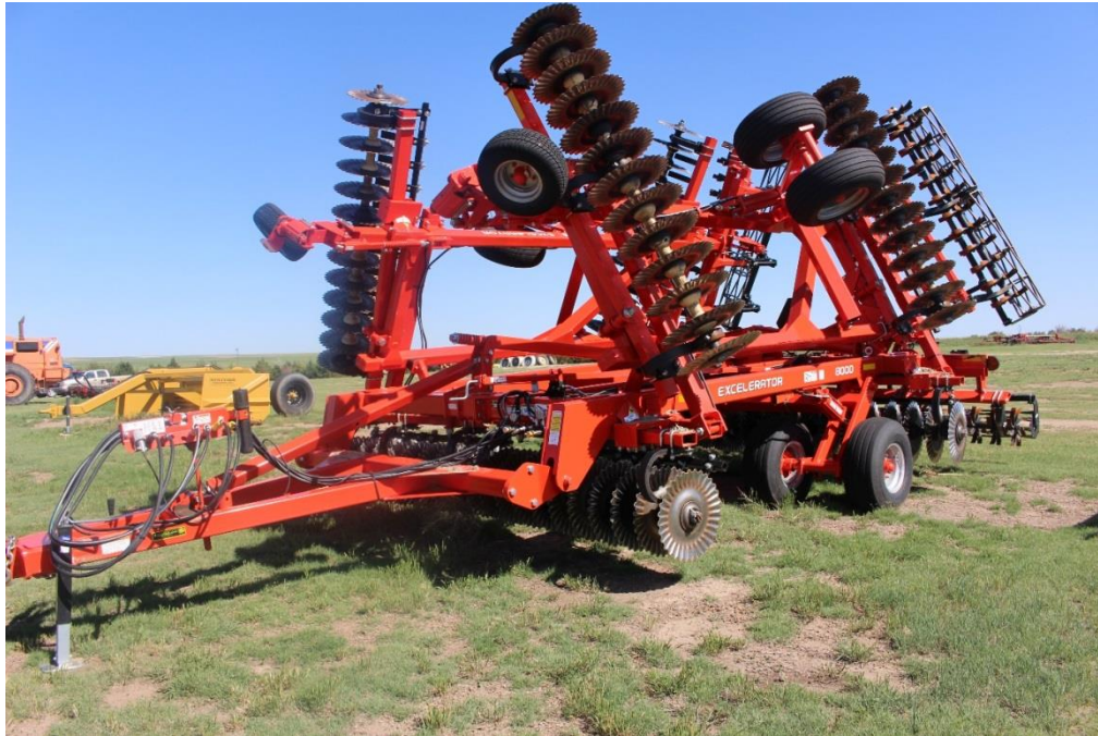
Figure 31. A typical vertical tillage machine as used in Kansas
