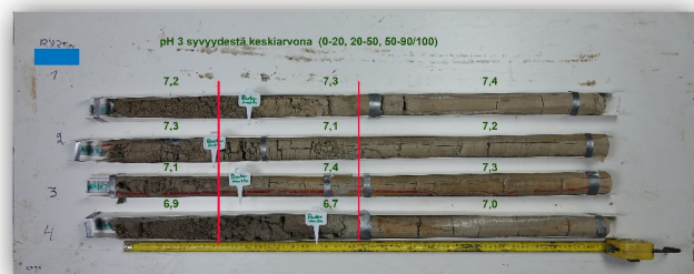
Amount and depth of SOM varies even inside the field boundaries. To get reliable carbon stock data, we need RTK accurate sampling points.
