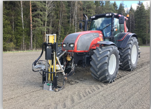
RTK-accurate reference sampling is important part of modern soil mapping. Sampling to subsoil depth is essential part of carbon measurement.
